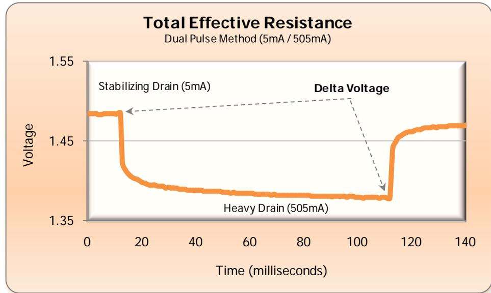
(fig. 9) 5 mA stabilization load / 505 mA pulse
